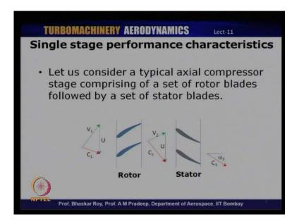
So, I mentioned that a combination of a rotor and a stator put together is a stage. So, this is this these put together constitute a stage of an axial compressor and this is what we shall analyze and see how the performance changes as the operating conditions of this particular stage changes.
