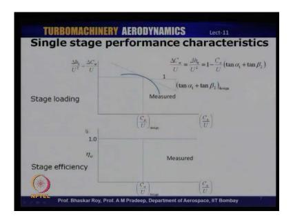
So, if I were to plot, let us take a look at loading coefficient first. So, I have loading stage loading on the y axis which is delta h naught by U square which is also equal to delta Cw by U. On the x axis, we have Ca by U which is the flow coefficient and we have seen this expression, we have derived this delta Cw by U is equal to delta h naught by U square is 1 minus Ca by U into tan alpha1 plus tan beta1.
