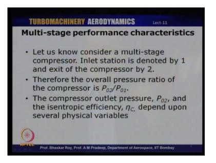
Therefore, the overall pressure ratio of the compressor, we will denote as P 02 by P 01 where P 02 is the compressor outlet pressure and P 01 is the compressor inlet pressure. So, the compressor outlet pressure P 02 and efficiency will depend upon several physical parameters or variables. So, we are going to look at what are these different parameters or variables on which the performance will depend. So, we will list all these different parameters or accompressor is going to depend.
