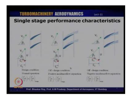
So, for that we have the velocity triangles for three different cases which have been shown. One is a design condition and two off design conditions. The design condition which is normal operation, we have Ca by U is equal to Ca by U design. This is the rotor blade and we have flow entering the rotor at an angle of V1 which is relative velocity at an angle of beta1.
