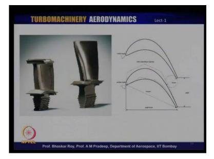
So, as you can see here in this picture. It shows that it is of a different color, because it is made up of very high temperature material, high temperature gas from the combustion chamber is going into the turbine. But these turbines are also made up of aerofoils slightly different kind of aerofoils, but indeed they are aerofoils and those aerofoils kinds are shown over here, on the right hand side.
