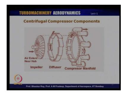
So, I am showing you here, a typical centrifugal compressor, which also does the job of compression and this flow here, it enters over here, it goes out from this side and then its surrounded by a row of diffusers, which is indeed equivalent to the stators that we talked about for actual compressors and when you put them together, the diffuser and the impeller together, you have a compressor.
