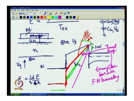
So, what happens when you start applying positive voltage as you can see here positive voltage will start accumulating the more and more electrons here correct that is a accumulation condition.
