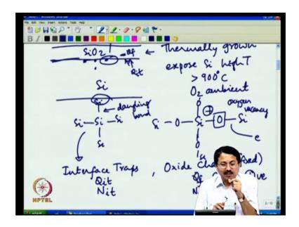
Out and it gets positively charge and this is what is suppose to give rise to all the positive charge that we see in silicon oxide at very close to this interface, and this is fixed because this is little bit away from the interface what you do in the channel has no bearing on changing this because you cannot have this carriers go in and change its state that is why is called fixed.
