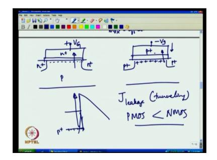
Remember n channel transistors have p type substrate and n plus poly silicon and they are mostly operated with positive gate voltage correct, that is we are interested in this kind of a tunneling, we have a positive voltage when you invert this transistor with the positive voltage there are lot of electrons. And these electrons can actually tunnel through. So, the barrier height here for electrons tunneling is what is important.
