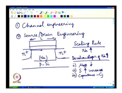
And the other one is source drain engineering. Based on our discussion so far, it has become clear that if we want to design a very small geo metric transistor. This particular case we are looking at n channel transistor.
