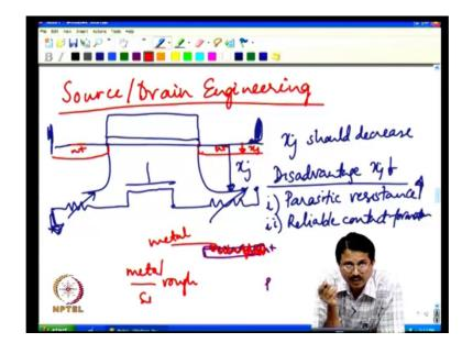
So, this is what we mean by channel engineering. The next important aspect is, the source drain engineering. So, again here what does the scaling theory tell you? This is the junction depth, with technology generation scaling; this xj should decrease, very obvious.
