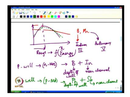
So, todays transistors really use a combination of, for example, if you want to do a p well, p well is what is required to define n channel transistor, this is for n mos. Use a combination of boron plus indium, and boron is defined, used to define depth of the well, ok.
