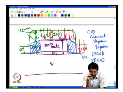
What is done essentially is that, you have the silicon wafer, you already defined this gate. Gate is defined using photolithography you see, depending on what is the length and width of the gate, you have printed that already. This is SiO 2, and this is gate; either poly silicon or metal depending on which technology you are your looking at.
