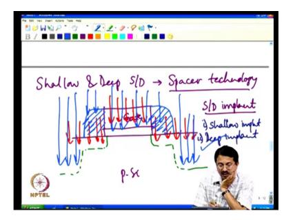
This is realized, the shallow and deep source drain, is realized using what is called spacer technology. What it means is the following you see. One is to get these junction energy, but just as I mentioned all the impurity introduction is done using implantation.
