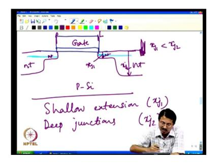
So, this is where I do what is called source drain engineering. So, in other words when I built source and drains of the transistors ideally I would have like to build a very shallow junction, which would look like this, but there is going to be lot of problems with this kind of a shallow junction. What I do. I do via media; I do something which would look like this.
