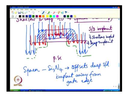
So, the spacer typically is silicon nitrite, and it offsets deep source drain implant away from the gate edge; that is the whole idea. So, at the gate edge, where it matters shallow junctions, you will retain shallow junctions, but away from the gate, defined by the spacer thickness you have deep implants. So, this is essentially done, you know with the series of you know some very simple, but very intelligent process steps.
