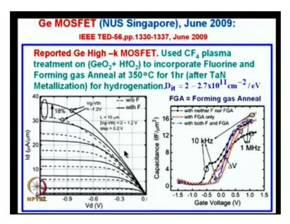
For germanium MOSFET from NUS, National University Singapore June 2009 transaction (Refer Time: 15:44) this picture is taken from there 2009. Germanium high k MOSFETs using CF 4 plasma treatment, germanium oxide plus hafnium oxide dielectric
