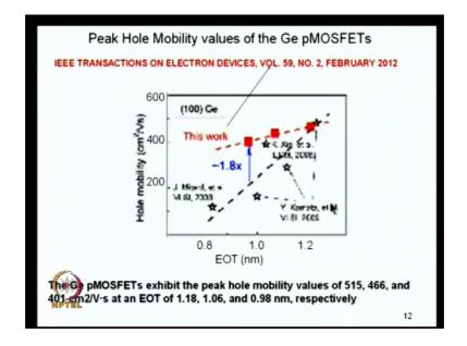
And they also measure the mobility from this I V characteristics, estimated the mobility and they showed that the germanium p MOSFET exhibit the peak hole mobility values of 500 and 15 centimeter square per volts second when the EOT of 1.18 is used there. EOT of 1.18 that gives about 515 that is highest ever reported for germanium p channel MOSFET.
