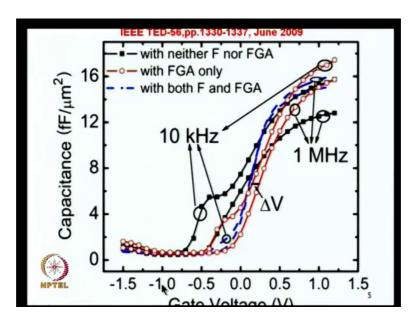
These are the capacitance voltage characteristics taken on these devices for example, just only the germanium thermal oxide and hafnium oxide and tantalum nitride and with only PDA, no forming gas annealing, no fluorine passivation. When they did that this black squares show the C-V characteristics at 1 megahertz and this upper curve shows the frequency response in 1 kilohertz.
