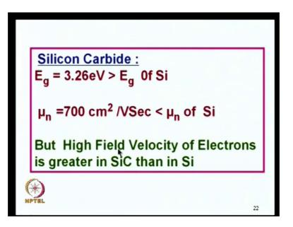
Now silicon carbide 3.26 electron voltage is a band gap higher than that of silicon fine, mobility is very poor even half of that of silicon less than that of electron mobility in silicon. But it will be high field velocity of velocity of electrons will be high at high fields that we will see later.
