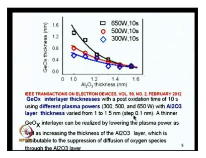
What they saw was they are able to control the thickness of germanium oxide you can vary it from 0 to 1.5 nanometers either by fixing the aluminum oxide for a particular thickness say here fix it at 1 nanometer Al 2 O3. Then subject it to that oxygen plasma at 300 watts you get about 0.5, 0.6 nanometer germanium oxide. 500 you get more oxide, 650 will they get about 1.3 or 1.4 nanometer, so if it 1 nanometer fixed more power you get more oxygen atoms diffuse through the Al 2 O3 layer.
