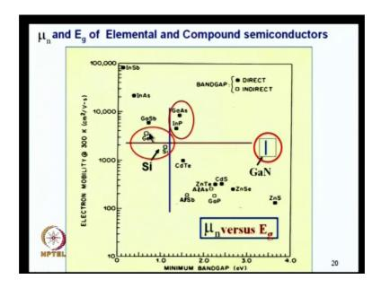
So, this is the famous graph which gives you electron mobility at 300 Kelvin on the y axis 100, 1000, 10000 etcetera and on x axis the band gap. Minimum band gap meaning actually energy band gap actually, because there are different band gaps but the minimum band gap is that the actual band gap.
