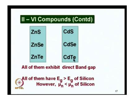
Now 2-6 compound as already mentioned, zinc sulphide, zinc selenide, zinc telluride, cadmium sulphide, cadmium selenide, cadmium telluride. All of them exhibit direct band gap because of their nature of heavy atoms without getting into the peaks of that the high atomic number elements from their compounds usually they turn out to be direct band gap that is an observation it is all.
