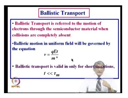
What is ballistic transport? Normally the electrons get accelerated they get scattered to collisions with lattice atom or impurity ions everything whatever it be waving scattering centers.
