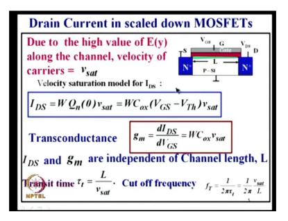
Due to the high value of electric field in the y direction, that is along the channel length the velocity of carriers will be saturation velocity.
