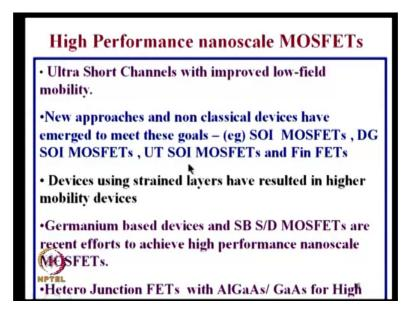
So, to get high performance what should you do? We just last time which I am discuss here today which has per lot of juice in that high performance nanoscale devices therefore, should ensure the doping is low. So, that mobility is high they should also ensure that the vertical normal electric field is low. So, that again the mobilities low field mobility is high ok.
