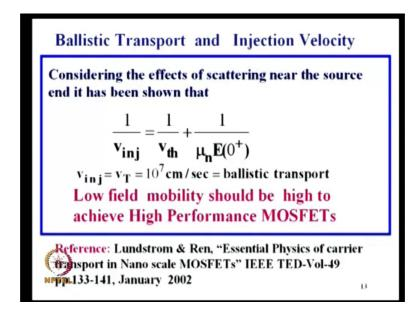
On the physics of carrier transport in nanoscale MOSFETs published in January 2002 in which what they have said is, what the carriers are injected from the source to the channel. They are able to inject from the source to the channel by gaining an energy to raise above that barrier ok.
