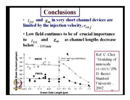
It is particular term drain current that you gets saturation drain current will be in the very short channel devices are limited by the injection velocity, which is controlled by both saturation velocity or thermal velocity and the mobility and you can see that both the terms which determine the injection velocity are independent of the channel length.
