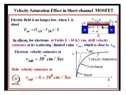
Now if you take a look at the velocity saturation effects on the short channel MOSFET what will be the electric field? The electric filed along divide direction that is from the source to the drain in that region, there is a voltage drop equal to gate voltage minus
