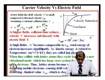
Now, before we go into that velocity saturation, we take a quick look at the velocity versus electric field characteristics of the carriers. I used the word carriers because the
