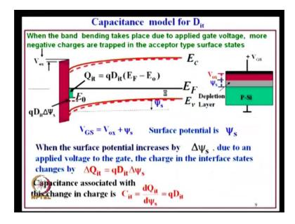
Now if that gate voltage is changed by delta V G, that delta V G will be shared between the oxide and also psi of S that diagram we have drawn here. I have increased that V G by delta V G. So, due to that there will be delta V oxide addition what so voltage drop delta psi of S, silicon voltage drop changes by delta V silicon or delta psi of S.
