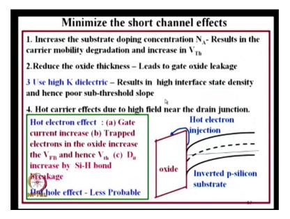
Now, the last 1 that I wanted to say here is the sum up short channel effects I know that I am re doing stating what was done earlier, you need to increase substrate doping concentration to reduce the short channel effects that results in carrier mobility degradation and increase in threshold voltage. To reduce you have to reduced the oxide thickness to overcome this effect but this of course, leads to get leakage current when you go to nanometer level.
