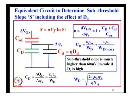
Now what will happen originally interface state density was equal to 0, we found out the sub threshold slope S equal to n V t lon 10 and n was equal to 1 plus C D by C oxide. Now when you change the delta V G the charge change was only across the C D because of the widening of depletion layer.
