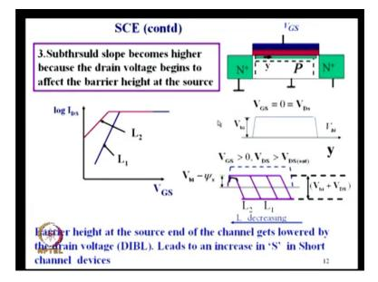
Now, I just wanted to bring in this the other effected during induced barrier lower this also have been discussed, I just drawing what happens here in the sub threshold region. In the sub threshold region there is no drop across the channel because the carrier there is
