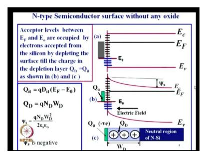
Now I will take a situation where see here it was a situation where it is a P type, Fermi level doping adjusted, bulk doping adjusted such that Fermi level is coinciding with the E naught. Now I go to a N type material doping something is like 10 to the power 15, or 16 Fermi level close to the conduction band decided by the shallow donors. Now surface is free there are no oxides, there are very large density of states.
