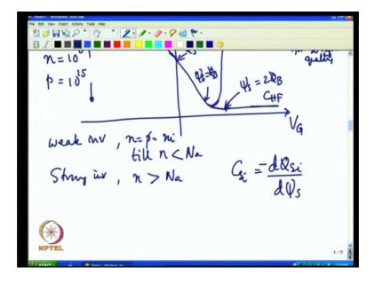
Silicon capacitance is d Q silicon divided by d psi s of course, this is a negative sign this is how I defines this when I change the surface potential a little bit what is the charge that is coming here and I did mention that in inversion the charge is dominated by the electrons majority I mean the.
