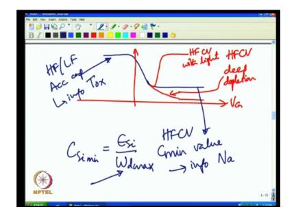
It is like photo vortex right you have a light you generate electron hole pairs when you did not have any light that is a thermal equilibrium you know given the room or whatever ambient temperature of the measurement that temperature has thermal generation the generation is only due to the ambient temperature, but if you have a light you will again get erroneous capacitance and it is important to do a high frequency measurement.
