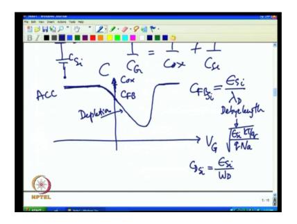
So, all it means is that if I now where to look at the capacitance voltage curve this is telling me this is a P type V F B is 0 flat band condition at 0 gate voltage and that will have some capacitance. In fact, it turns out we call it C F B flat band capacitance we will come to the definition of flat band capacitance in a minute for negative gate voltages on a P type substrate we are accumulating more and more hole right negative gate.
