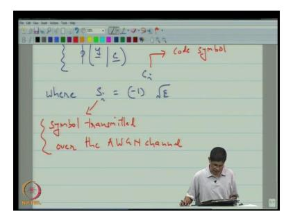
When round the channel module here, I put down input s which is plus or minus, but or coders always been 0 or 1. How do you make the connection; the connection is enough, where S i is equal to minus 1 to this c i times root E this is the nothing, so this will be here is the code symbol whereas this here is the symbol transmitted. You know the clear that talk let us see if can with more information about the decoded.
