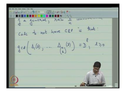
So, the analysis result propagation rate k by n code and going to actually, put that down. Theorem analysis putting bracket CEP, a necessary and sufficient condition on the P G M of a general rate k by n convolutional code to not have case tropic error propagation is that the GCD of delta one of D comma delta n to is k of D is equal to D to the l for l greater than or equal to 0.
