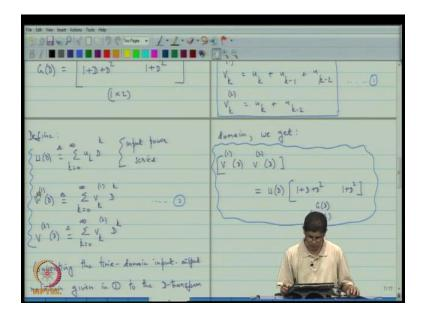
So, on the left what we have is the polynomial description of the encoder; and this is be called, polynomial generator matrix. And the input, output relationship is in terms of power series. So, there is the power series that represents the input, and there are two power series that represents the output, because in this case, the convolutional code has one input and two outputs.
