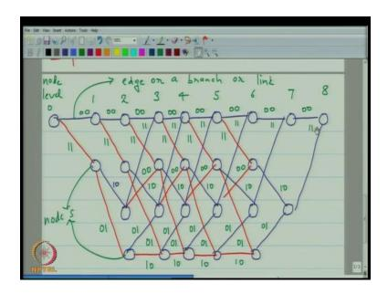
Here, I have the trellis and I am going to move it. Let us paste here labels and now, what I am going to do, thus the missing state is put that in. So, one terminology is that of nodes and so, every one of these is a node. So, let me use the different color for this, so these are nodes in the diagram. What you see vertically across time here, these are node level, so this is node level 0, 1, 2, 3, 4, 5, 6, 7, 8 and these corresponds to different instance of time.
