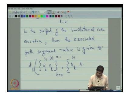
So, maybe I should to this put down few notes, corresponding to some of the terminology and introduce here, if v k 1, v k 2, k goes to 0 to m minus 1, where m is less than or equal to n, is the output of the convolution encoder, then the associated metric. The associated, the path segment metric is given by the hamming weight between and the corresponding receiving sequence.
