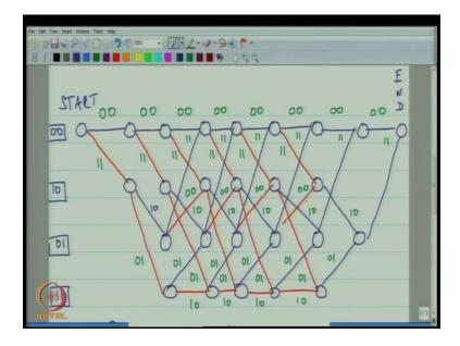
Then, we went on to talk about the state diagram of the encoder, viewed as the finite state machine, and then we started drawing the trellis diagram. And as I think I mentioned last time,
