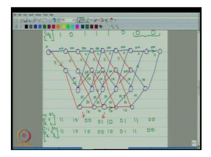
Let us select the trellis and copy it of few times over. I got the trellis copy, the few times. I can form the trellis from 1, 2, 3, 4 and go back on this 1. Now, so then, but I want to do is I just illustrate the input sequences. Here, putting this, the rarer dark or just to dark. Let see how do we want to do it, maybe I will try, to put in arrow, along the paths. So, let us put this is 1, this is 0, this was 1 1; so let two 1s, three 1s, and have three 0s.
