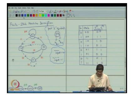
And then we drew the finite state machine diagram, for the convolution code, which directly relates to the state diagram that actually see you over here. We looked at the finite state machine, and this is the table that tells you that if you are in a given state, in have given input, what is the output? We have labeled the diagram according to that; they started drawing the trellis is to give the idea.
