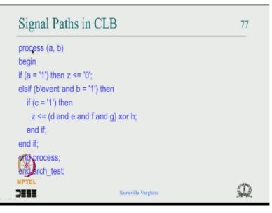
And we said it is a process a is reset, b is the clock, c is a control signal and z is d and e and f and g and xor h. We have discussed this will be a 2, 4 input lookup table cascade, c go to the enable clock of the flip flop, d is a path a reset ok.
