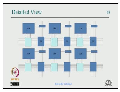
And this is the main you know the wiring diagram you have main switches and this is the logic block and this input to the logic block output from the logic block.
