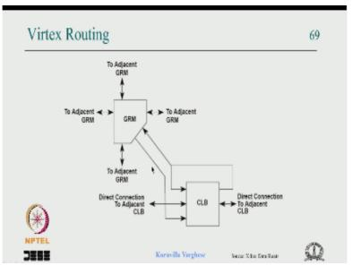
As a picture shows that are directors running from this switch to the CLB and the adjacent CLBs are connected with dedicated wires that means this CLB output can go to the input of the CLB and this CLB will be received input from the CLB output without going through the wire. So that can be very fast.
