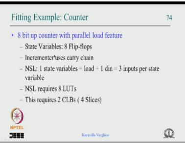
And we have looked at the 8 bit counter with parallel load features, so this is the count of the 8 flip flops with the +1 implemented and we said that this look up table with the carry chain can implement +1 and flip flop. So the 8 flip flops and 8 bit lookup table with a carry chain that requires. So it is basically it requires 2 CLBs.
