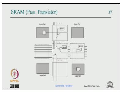
And we said that the SRAM basically used a transistor and NMOS transistor for interconnecting the two wires but then at the gate is like NMOS, the gate is 1 it makes a connection gate is 0, it cut off the connection ok, now the gate is a flip flop which holds that that status of the connection if the flip flop is set to 1 then it conducts if it is 0 it does not conduct.
