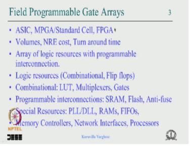
But in FPGA the interconnection is with programmability built into the gate, this Array Logic resources, so that it can be programmed or configured in the field. So the game is between the NRE course which is very high for ASCI medium for this and low for this. So this ASIC workout for huge volumes and this for middle volume and this for low volume and the design turnaround time very high for it and low for it.
