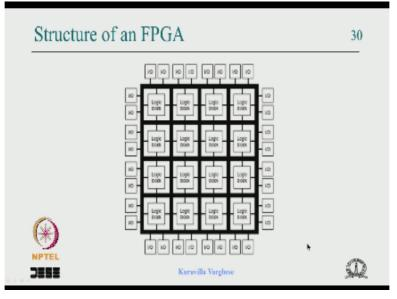
And also processor, so this is general structure of FPGA, I/O pins around, array of logic blocks normally this will run into 10s and 100s okay like across and across the row and across a column, ok that this may be typical numbers will be for small 150 by 52 maybe 100 by 100 it may go all the way to huge numbers ok and that shows that you cannot interconnect those blocks with a single switch.
