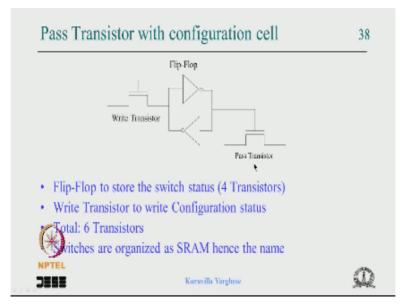
So but one issue with the SRAM is that this is a simple flip flop ok. So you look at this whole block ok. Now I hope you remember that this is a logic cell, this is a logical cell, these 4 are logics and these are those are the horizontal wires, these are the vertical wires to get whole interconnection at this big switches and output interconnecting to the to the vertical wire ok, just an explanation on the diagram.
