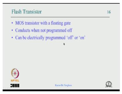
And when it comes to MOS transistor we have seen that with respect to the PLDS, CPLDs and MOS transistor has a it is a normal MOS transistor with the floating gate it conducts when it is not programmed of and can be electrically program off or on.
