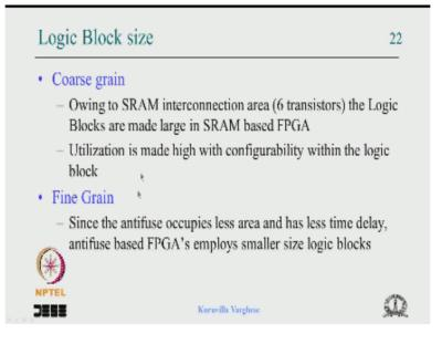
So this is one important things though nowadays most the complex FPGAs are SRAM. (Refer Slide Time: 29:11)
