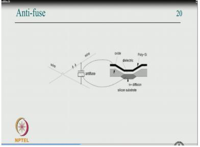
And the third one is call anti-fuse or anti-fuse and you know that in a chip design you have layers which implements transistor and your have layers with interconnecting wires ok. So you cannot have the wires in the same layer of the transistor. So there on a different layer and the layer to layer connection is by drilling a hole and normally on one layer the wire run horizontal in the next layer.
