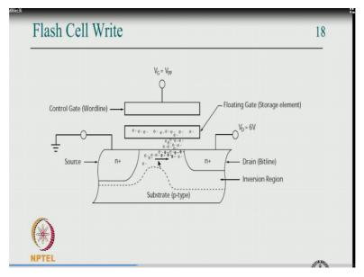
So that makes it off you know you apply the control gate with logic high it does not conduct, so that is how it is turned off so that is shown here, the source is grounded drain is given the supply voltage pulse is applied a higher voltage power supply electrons and getting here and then the normal application of the gate voltage would not make the channel and it would not connect.
