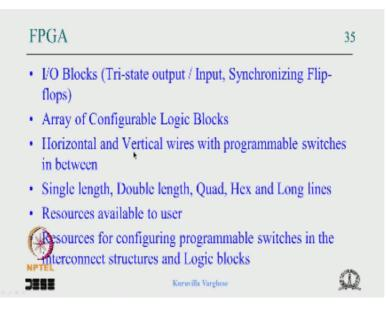
So FPGA comes I/O blocks and that has tri state output and input and it has synchronizing flip flop because the input can come from another chip for another clock domain and array of configurable logic blocks, the horizontal vertical wires with program which is in between these wires are single end, double end, quad, hex and long lines, it depends on as a statistic or how statics the circuit of the connection.
