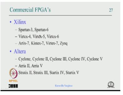
And also that is filed programme of get natural we have seen commercial FPGA Spartan and Virtex from Xilinnx and cyclone and Stratix and area from Altera.
