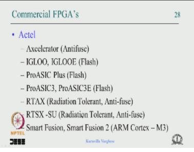
And Actel has this ProAsIC and accelerator and radiation tolerant version of the accelerator smart fusion with Arm cortex and things like that and of course as I said the Xilinx Zynq with dual core RAM and the Altera has soft core.
