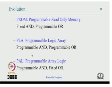
The next one was at this AND was an overkill because in a chip select decoding very few AND gates are usually 1 AND gate is used even in real Boolean functions number of products or min terms are less. So we reduce the number of AND gate but then it necessary rated to make it Programmable that means increasing the number of inputs to 2n and which is program and that enable not only them min terms of the product which was much more kind of use, if it allowed to reduce the number of the AND gates.
