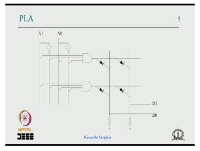
So that what we said we can reduce and get but the AND gates should be programmable the minterms become the product comes and such a device was PLA okay. The Programmable logic array it was called, it is called programmable logic array ok that I am not written that in the previous slide.
