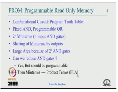
You can implement a combination cute essentially you program the truth table and we have seen that it is a fixed and it is a programmable OR ok. The AND is fixed by the storage to an AND gate in the case of any input by blowing or retain the fuses are we are programming 0 or 1, so you can you are able to program the truth table and also like when in the case of multiple outputs multiple like in this case 2 output same minterm can be chosen ok.
