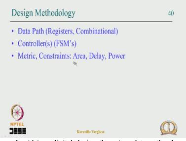
So let us continue as I said in a digital design there is a data path where the computation happens it is made of registers and combination circuits. Registers holding the value, combination circuit computing it and there are controllers are finite state machine which control the data movement in the data path, there could be multiple controllers or single
