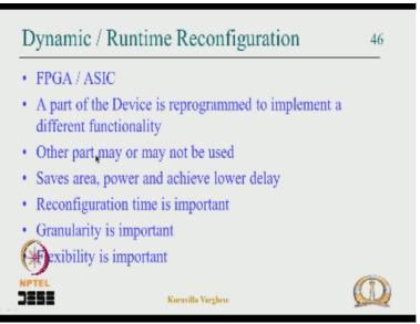
So let us move on this is the next technologies that is something called dynamic or runtime reconfiguration which is very much talked about research pretty much. So this can walk in FPGA and ASIC level and the basic idea is that a part of a device reprogram to implement a different functionality, that means take an example say you have a SOC which is used in a mobile phone and suppose you are working with bluetooth ok.
