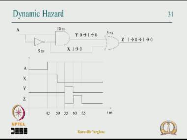
You can have dynamic website for a single change in the input that could be multiple glitches at output instead of 1 pulses.
