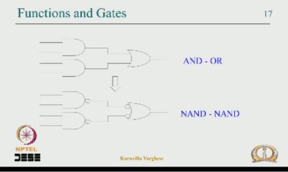
We have seen some example of AND OR is getting implemented using NAND-NAND gates and also we have seen how advantages is to conceptually thing like that then you will not raise gates if you bring this in the concept while designing some simple logic circuits.
