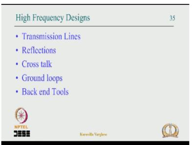
So that is high frequency design you know that in high frequency the tracks or the lines of the wires within on a PCB or a chip can act like transmission lines. So there could be reflections, so unless we take care maybe your logic is correct, the timing is correct, everything else is taken care, but because of the high frequency the wires can act like transmission line. If there is impedance matching problem there can be reflections which can corrupt the signal.
