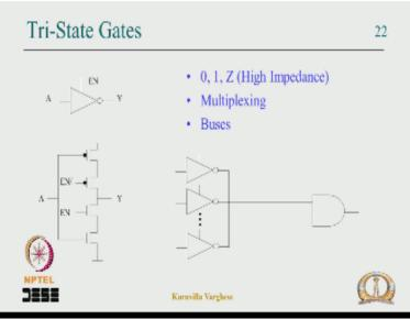
And we have seen what is Tri-state gates and some care I need be taken when you are bussing or multiplexing using the Tri-state gate or pull up pull down.
