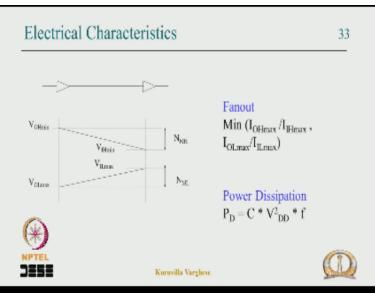
Then we have seen the noise margin the fanout, how to calculate the fanout, the power dispassion in the power for switching, power dissipation, power dissipation leakage, power dissipation expression for the power dissipation in CMOS output stage.
