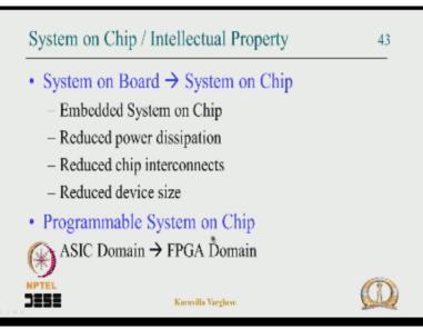
But things are singing the complete system for me on a chip, it will reduce the power dissipation, reduce the area, the cost will be reduced, the delays will be less and the power dispassion will be less. And same thing is happening in the FPGA dominos also. In the ASIC domain a system on board, in the FPGA domain you have Programmable system on chip ok, that means you have in the FPGA domain also.
