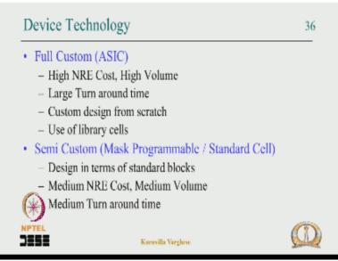
So let us move on to the next technology that the device technology. So our courses about PLDs and FPGAs. So it is let us have a look at what are the device technology available, one thing is the application specific in the greatest circuit or ASIC and this is normally supposed to be full custom. So the that means it is design from scratch you know almost everything is the sign at the gate or flip flop level.
