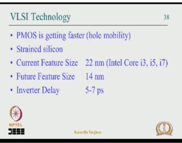
So the next I want to search on the current state of the VLSI technology, you must learn that the PMOS is slower than NMOS. Because the whole mobility in PMOS is less than the electron mobility in NMOS. But you know that the current technology like strained silicon the PMOS is getting fastest. Strained silicon means a silicon lattice structure is strained by some deposit on top of silicon.
