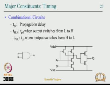
We have looked at the timing that is a second important constituent of the design and for combinational circuit what is the timing, it is a propagation delay.
