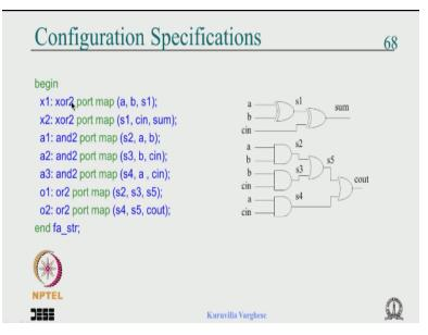
You say x1, x2 are the xor gates. You can see it is nicely instantiated abs1 s1cin a sum and2 is kind of reverse so, ab and s2 bc and s3, bc and s3, ac and s4 that is the and2 and or the first or is s2, s3, s5 that is this and s4, s5 cout that is this. Now we are going to say where the x1, x2, a1, a2, a3 o1 or2 is coming from so, we have mind you we have 2 xor gate, 3 and gates and 2 or gates okay, x1, x2 a1 to a3, o1 and o2.
