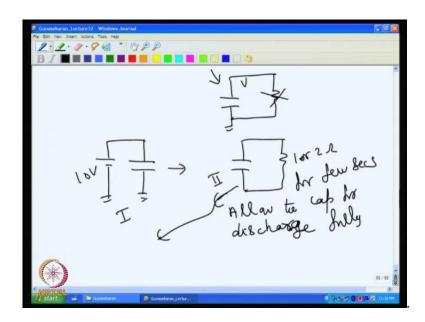
Even though the capacitor temperature drift and long term is not a issue, the dielectric absorption of the capacitor is the major issue, so the dielectric absorption of the capacitor
