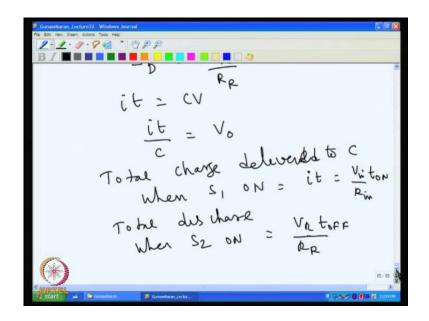
So total charge during S 1 on was total charge, total charge delivered to C when S 1 on is equal to i into t and then that is equal to V in by R into t.
