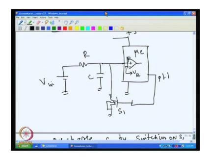
Now we can have for example, because many of the micro controller have inbuilt comparators, we can have this if it have been given to the input comparator and the V reference this given to the V Reference.
