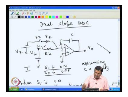
So that V 0 is coming as V in by R in is i into t divided by C that with minus sign, so it goes minus side, so the minus sign is introduced to take care of the inversion. So we will take this that is the equation for V 0. Now what is that it signify that is, if I have the input voltage I make the switch on for some time, the switch S 1 on for some time and then I will I will see that output voltage increases with time, there output of the op amp
