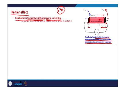
A complementary thermoelectric effect is the Peltier effect. And what is Peltier effect? It is the development of temperature difference due to current flow in a conductor ok. And now we need to be very careful because due to current flow the heat is generated because the joule heating is appears because of the current flow because of the scattering of electrons with the lattice atoms or intra or in electron-electron scattering
