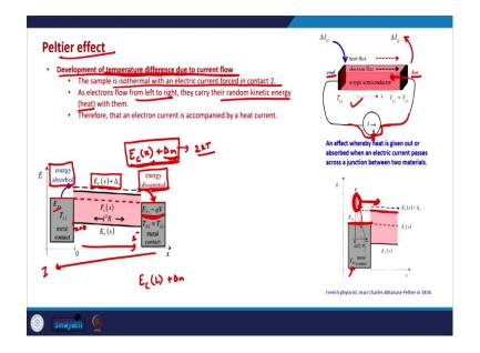
And in this case initially the sample the semiconductor is isothermal, which means the temperature is the same everywhere. And electrons as electrons flow from left to right they essentially carry kinetic energy and what it means is that they carry a certain form of heat or they carry heat in the form of kinetic energy from left contact to the right contact.
