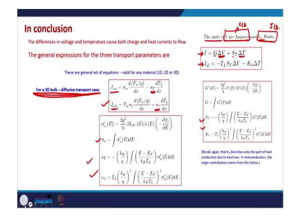
So, in conclusion what we can say is that always the electric current the charge current and the heat current are accompanied with each other and both of them depend on the applied voltage and applied temperature gradient in the system. I would also like to say that just to sort of remind you that the Peltier this temperature difference due to current flow this is different from joule heating.
