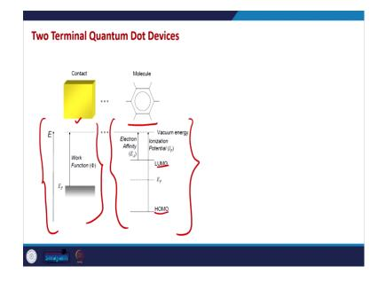
So, what happens when we put a metallic contact in touch with this molecule or quantum dot? So, on one side on the metallic side electrons have this kind of energy profile on the right side in the molecule in the quantum dot electrons are like this on the left side they are in a continuum of energy and the occupancy is governed by the Fermi level. On the right side they are in discrete energy levels and occupancy depends on the number of electrons in HOMO and LUMO orbitals ok.
