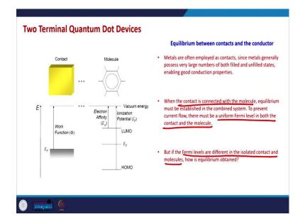
So, it is interesting what happens when these two are combined when we put a quantum dot in touch with the metal in equilibrium what happens is when a metal is connected to the molecule.
