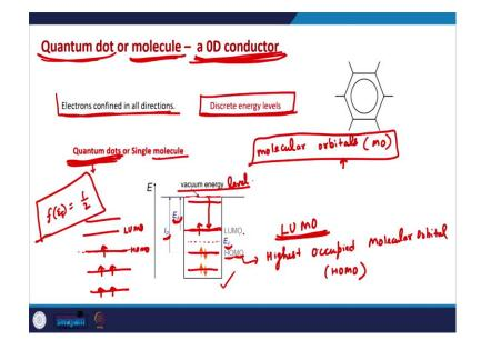
So, now let us begin with the quantum dot devices, a quantum dot device means that the active region of the device now is a quantum dot or a 0D conductor, which means a conductor in which electrons are confined in all the directions ok is. So, it can be a molecule it can be a nanostructure very small nanostructure in which electrons are confined from all the directions.
