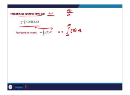
So, in order to understand the effect of charge transfer on the Fermi level we essentially need to calculate this quantity how does the Fermi level changes with respect to the change in charge. And this will come from this relationship, which is the relationship between the number of electrons to the Fermi function.
