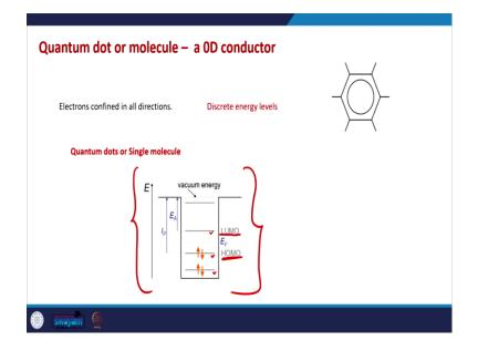
So, that is a; that is a very general model of the contact and just to quickly remind you a general model of a quantum dot or a nanostructure or an organic molecule or any general structure that is in which electrons are confined in all the directions is this in which we have molecular orbitals.
