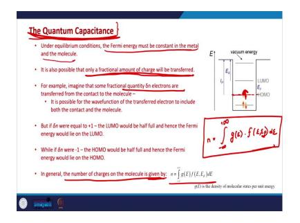
So, let us first consider the what is known as the charge the state filling effect which means how does the Fermi level depends on number of electrons in a system because whenever we put a metal in touch with a quantum dot the number of electrons will change in both the systems.
