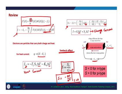
So, what we have seen is that that in the expression of the current  $(f_1 - f_2)$  is the forcing function. And forcing function means that, if this term is non zero in that case the current will be will also be non zero. And  $(f_1 - f_2)$  depends both on voltage difference across a conductor and temperature difference across a conductor.
