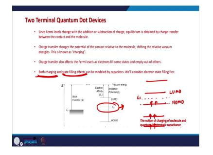
Because if the number of electrons in a quantum dot let us say if we have a quantum dot whose molecular orbital are organized in this way. If the number of electrons in this system are just 5 this becomes the HOMO orbital and this becomes the LUMO orbital and the Fermi level lies at HOMO.
