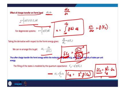
The way the reason we can write it like this is that generally, the Fermi level of the metal does not change with the change does not change with the number of electrons because there are already a lot of electrons in the metal. So, even if few electrons go to the contact or few electrons come from the contact the Fermi level does not change much. And generally the equilibrium Fermi level is at the Fermi level of the metal and that is why this integration limits boil down to this level.
