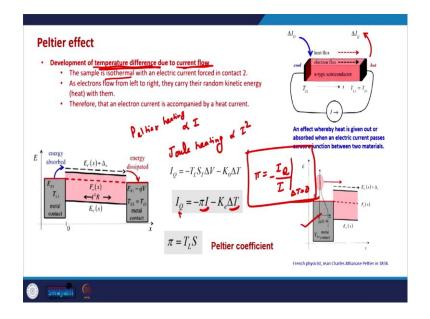
And in other words what it means is that if there is no temperature difference that we do not apply any temperature difference we take an isothermal conductor. So, if this  $\Delta T$  is 0, in that case  $\pi$  is or the Peltier coefficient is essentially the ratio of the heat current to the charge current essentially at  $\Delta T$  equal to 0. So, this is the definition of the Peltier coefficient and as you might have already guessed the Seebeck coefficient or the Seebeck effect.
