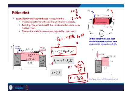
So, now we need to understand the heat current and the heat current is given by if you remember from the last class is given by this expression  $I_Q$  is  $-T_LS_T\Delta V - K_0\Delta T$ . And this is rewritten as this term  $I_Q$  is  $-\pi(\Delta VG) - K_0\Delta T$ , ( $\Delta VG$ ) is the current the charge current in the system because of the applied voltage. So, this becomes I. So, that is why we can write it like this.
