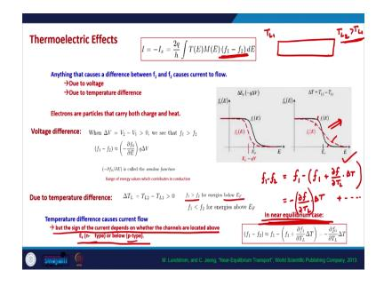
Now, because of the temperature difference, now  $\Delta T_L$  is  $T_{L2} - T_{L1}$ . So, here we have  $T_{L2}$  we have  $T_{L1}$ ;  $f_1$  is greater than  $f_2$  below  $E_F$ ,  $f_2$  is greater than  $f_1$  above  $E_F$ . So, as I just told you that depending on if the channel is n type the what happens is in n type channel conduction happens because of the electrons in conduction band.
