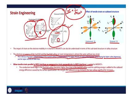
So, let us try to understand it in a more physical way. So, this is the unstrained silicon and in unstrained silicon MOSFET as we have already seen because of the quantum confinement there is energy splitting.
