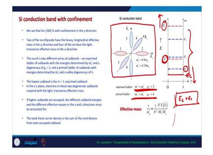
So, the all almost all the MOSFET theory will be the same. Here instead of  $E_C$ . So, this is the bottom of the conduction band instead of  $E_C$  we need to consider  $E_C + \notin 1$ .
