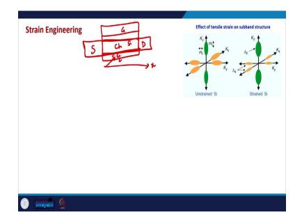
Please remember that the direction in which the stress is applied or the strain is applied is extremely important and this is the case of biaxial strain. What it means is, that if this is our MOSFET let us say this is the source, this is the channel, this is the drain.
