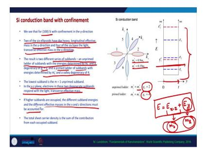
So, in both the cases we need to consider the quantum mechanical nature of this confinement. So, if we take a 100 silicon wafer by 100 silicon wafer we mean that the surface of the wafer is in this plane actually.
