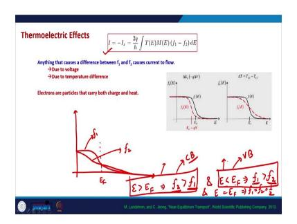
Let me redraw it this is the let us say the Fermi level at Fermi level, the Fermi function is always 1 by 2. So, that is what we will do and if the temperature is increased this is how it looks like. So, what happens is that this is  $f_1$  which means, Fermi function at  $T_{L1}$  and this is  $f_2$  the Fermi function at  $T_{L2}$ . So, for energy is greater than  $E_F$  above Fermi level  $f_2$  will be greater than  $f_1$ .
