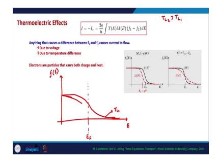
The way the Fermi functions will be modified is, the Fermi level would not change in this case. So, the Fermi level will be the same we are plotting Fermi function as a function of energy and at temperature  $T_{L1}$  let us say the this is how the Fermi function will look like. So, this is  $T_{L1}$ , ok. If  $T_{L2}$  is more let us say  $T_{L2}$  is greater than  $T_{L1}$  in that case this Fermi function will be even more broaden.
