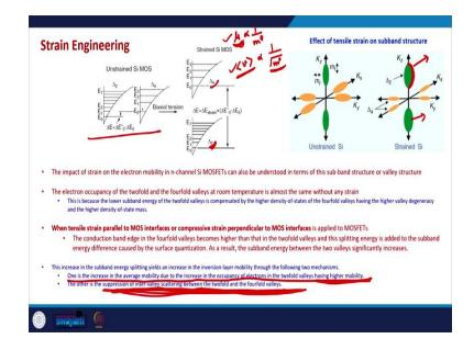
So, that leads to increase in the mobility or injection velocity of electrons in the channel and there are two reasons. One is the increase in the average mobility is due to the increase in the occupancy of electrons in the two fold valleys with higher mobility.
