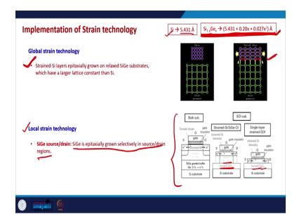
So, this is the way this strain technology is implemented. Generally as I already pointed out to you in order to make a silicon channel or make a strained silicon channel in order to make a MOSFET channel in which silicon lattice is strained in a specific direction.
