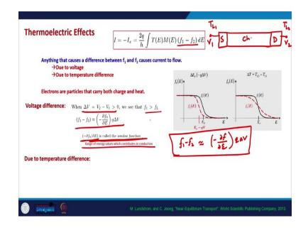
So, because of the voltage difference  $\Delta V$ , so let us draw this conductor again we have a source, we have a drain, we have a channel and let us say this is on V<sub>1</sub> voltage this is on V<sub>2</sub> voltage. This is on T<sub>L1</sub> temperature this is on T<sub>L2</sub> temperature. So, if V<sub>2</sub> is greater than V<sub>1</sub> in that case f<sub>1</sub> is greater than f<sub>2</sub>.
