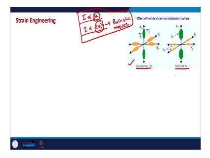
So, with this background let us go to the strain engineering in silicon and the strain engineering essentially means that, the device performance is enhanced by applying an a applying a mechanical strain.
