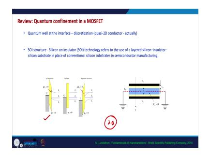
So, what we have been seeing is that even in bulk MOSFET there is a confinement of electrons in the inversion layer and in ETSOI structure this confinement is there because of the geometry of the devices. So, that is why we need to consider and this these, all both of these confinements are of the order of the de Broglie wavelength of electrons.
