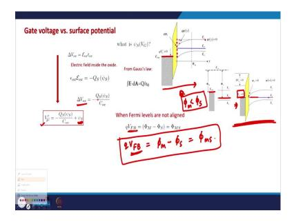
And so, that is why the gate voltage the total gate voltage is  $\Delta V_{OX}$  which is  $-Q_S/C_{OX} + \Psi_S$  which is the voltage that drops inside the semiconductor. And please note it down here that we have written a prime on V'<sub>G</sub>. What does the prime means here?
