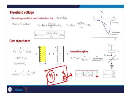
And that is  $\Psi_S$  is  $V_G$  divided by m. So, this m actually governs how much of the gate voltage drops across the semiconductor because if this m is close to 1 in that case  $\Psi_S$  will be almost equal to  $V_G$ . So, what we can say is that almost all the voltage drops across the semiconductor.
