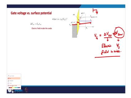
So, the one way to understand this is that, the voltage that we apply on the gate terminal is dropped in the oxide and in the semiconductor ok. So, the gate; because deep inside
