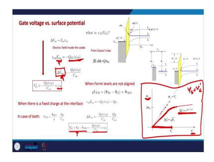
So, or  $V_G'$  is  $V_G - V_{FB}$  and this is given by this value. So, now, this is the relationship between  $\Psi_S$  and  $V_G'$ . So, this is a complex relationship I would say this  $V_G'$  and  $\Psi_S$  they are related to each other. Because this  $Q_S$  which includes the static charge and the depletion charge and the inversion charge this is a complex quantity, and then we have this  $\Psi_S$  term as well.
