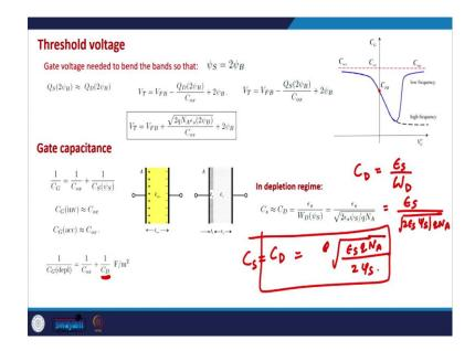
So, in the depletion region, generally the width of the depletion. So, in the depletion region what we can says that, the capacitance of the semiconductor will just be  $\mathcal{E}_S / W_D$  the depletion width, and the depletion width as a function of  $\Psi_S$  is  $\sqrt{(2\mathcal{E}_S\Psi_S/qN_A)}$ .
