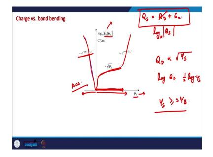
So, just to summarize all these various regimes, we can what we can do is we can plot a relationship between the semiconductor charge and the surface potential. So, the semiconductor charge  $Q_s$  is if you recall is the summation of depletion charge plus inversion charge, and in order to properly understand this we plot the log of the log 10 of  $Q_s$  take a mod as well we generally take a mod.
