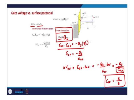
That in order to understand the relationship between  $V_G$  and  $\Psi_S$  we need to understand what is the voltage drop in the oxide and that depends on the electric field in the oxide. And in order to find out the electric field in the oxide we use the Gauss's Law. And what does the Gauss law says?
