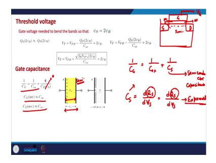
Let us quickly try to understand another important topic that is the gate capacitance. The gate capacitance is, essentially the capacitance of as seen from the gate terminal, and as we know that a MOSFET is also has a capacitive element. So, this is the gate terminal, this is the oxide and this is the semiconductor.
