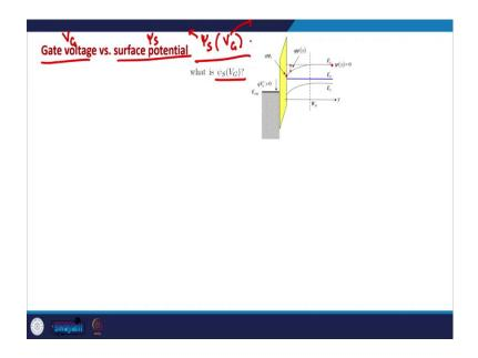
Now onwards we will try to see the relationship between  $\Psi_S$  the surface potential and  $V_G$  because  $V_G$  is the voltage that is in our hands. So, to start with what is that we are trying to find out? We are trying to find out a relationship between  $\Psi_S$  and  $V_G$  or we are trying to see how  $\Psi_S$  is a function of  $V_G$ , because  $V_G$  is the independent variable, psi S is the dependent variable;  $\Psi_S$  depends on the applied  $V_G$ .
