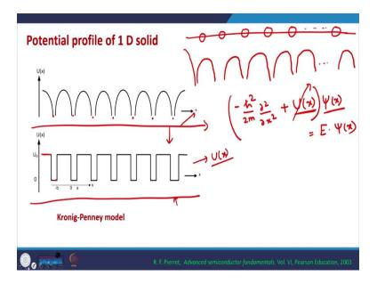
So, if we generalize basically this understanding this is how the potential profile or the to be more precise the potential energy profile of the electrons would be in a 1-D solid. So, in a 1-D solid if we precisely plot the lattice here the potential energy of the electron in this system would look something like this.
