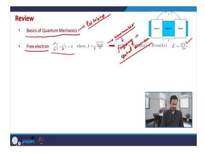
So, in the beginning I told you that the most important part of a device is of a field effect transistor is its channel. And the channel can be sort of understood as a two terminal device where we have a channel there is a source and there is a drain. And on application of a positive voltage on drain terminal electrons flow from source to drain. Now, as we know that in modern devices this channel region is getting smaller and smaller.
