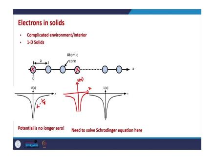
So, now let us see how it actually looks like potential due to atomic core due to let us say this atomic core is this as we can see this is basically the potential energy of the electron is inversely proportional to  $\frac{-1}{r}$ . So, the potential energy of the electron will be this, this is a graphical representation of the potential energy this is we are not.
