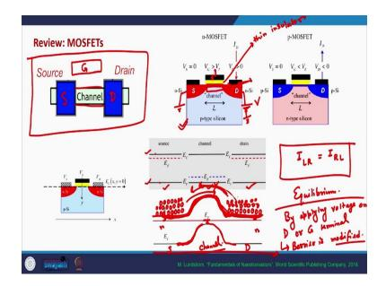
And that is easily visualized from the band diagram of the MOSFET. Let me quickly review, before going into the details of the band diagram, let me quickly review what we have been seeing. In this course in the beginning, we discussed this kind of a two terminal device, in which there is a source terminal, there is a drain terminal and in between them there is a small channel, ok.
