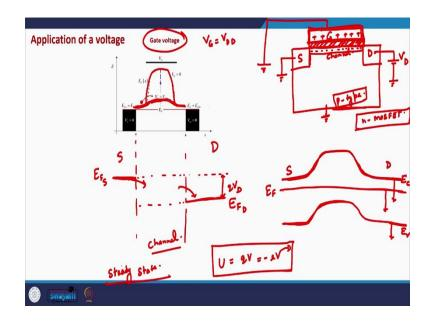
The Fermi level on the source side is this, the Fermi level on the drain side is; let us say this is the device, the Fermi level on the drain side is now lowered by the value of q timesV, that is the or  $V_D$ , if the  $V_D$  is the applied voltage on the drain terminal. So, this is source, this is drain, let us say this is the channel region.
