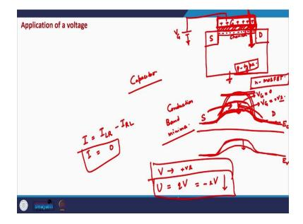
So, if we plot, if we draw this entire band diagram; this is the conduction band edge, this is the valence band edge. So, when there is no voltage on the gate terminal, this is how the barrier looks like; when there is a positive voltage, this will also go down.
