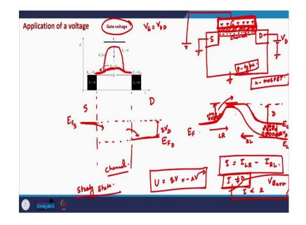
The current from source to the drain side will depend on the barrier height from the source side and the current from drain side to the other side will depend on the barrier height from the drain side.
