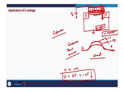
So, finally, we have a device like this; very simplistically we have source, we have drain, we have oxide and we have the gate terminal, ok. And the band diagram, equilibrium band, we just plot the conduction band minima. The valence band maxima will actually follow the conduction band minima exact in exactly the same way. So, the typically this is how
