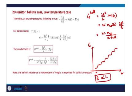
So, we have the conductance expression to be the ballistic conductances,  $\frac{2q^2}{h}$  M(E<sub>F</sub>) and M is directly proportional to the width. Let us say, W times M<sub>2D</sub>(E<sub>F</sub>) times  $\frac{2q^2}{h}$ . This  $\frac{2q^2}{h}$ . is 1 by 12.9 kilo ohms.
