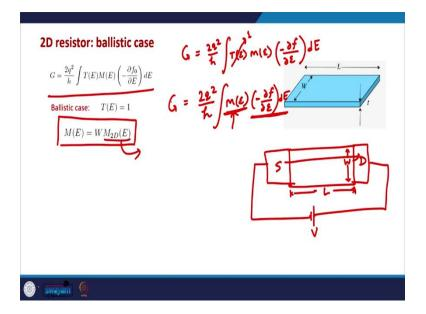
So, we have a 2D device let us say, the source, the drain, the length and width are there. And ballistic means that, the electrons are not colliding they are directly going from source to the drain side, which also implies that the length of the conductor is not large it is a small length.
