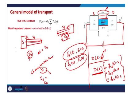
So, for example, if we are just considering the source contact and the channel at the moment we are not concerned about the drain contact. So, in this case the characteristic time of the source the  $\tau_s$  will be the time that an electron takes from the source terminal to cross the channel to go to the other end of the channel.
