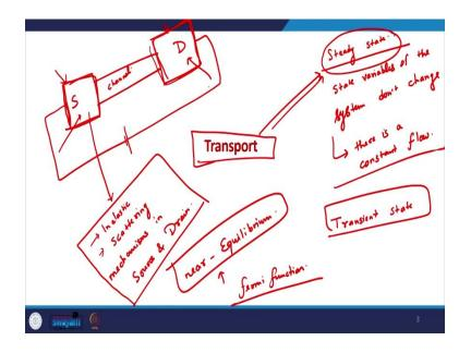
And there is a related concept of steady state; in steady state, also we can say that the state variables of the system do not change; the state variables of the system do not change, but there is a flow there is a constant flow so to say to be more precise there is a constant flow in the system.
