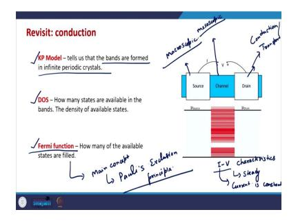
So, finally, we have this we have a two terminal device that we are trying to understand; we are trying to understand the mechanism of conduction or transport in a two terminal device and a two terminal device generally this middle region the channel region is taken to be a very small region the source and drain regions which are essentially like metals or which are like metallic contacts these are much bigger than the channel region.
