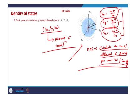
So, once we realize that the electronic wave functions in a 3D solid is a direct generalization of electronic wave function in a 1D solid, now there are allowed k values. So, the allowed k values will be like a 1D solid. These allowed k values will be  $k_x$  equals  $n_x \pi/L_x$ ,  $k_y$  equals  $n_y \pi/L_y$ , and  $k_z$  equals  $n_z \pi/L_z$ , ok.
