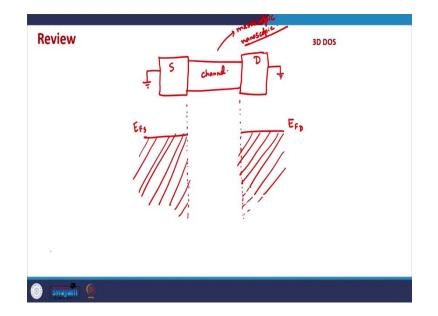
So, as usual we start with a two terminal device and a two terminal device looks like this. So, we have a channel region in between and on the left side we have the so called source contact, on the right side we have the drain contact. In this diagram, the channel region is shown as larger than the source and the drain, but that is not the case. Here it is drawn like this just for sake of representation, sake of understanding, so that we can understand things properly.
