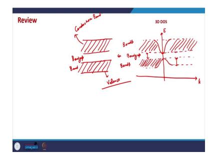
So, what we have seen so far is that because of the periodic potential bands naturally arise in solids, that is the conclusion from the Kronig-Penney model, KP model. And from there we saw that the E k relationship for a 1D solid and which can also be generalized to 2D and 3D solids, but it will be more complicated than the 1D case, this looks something like this.
