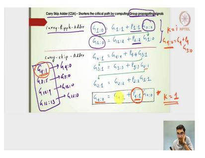
Let us begin with this, what we had seen is the carry ripple adder. Let me take the pointer the carry ripple adder. Here, the way we have utilized the group generate signals is  $G_{1:0}$  we generate it from  $G_{0:0}$  and then from 1:0 we generated  $G_{2:0}$  and then similarly we generated  $G_{015:0}$  for a 16-bit adder circuit.
