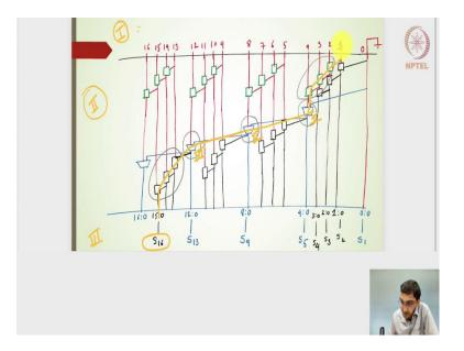
I will have a delay from this particular first stage which is nothing but the bitwise generate and propagate signals the delay due to that. The second one I will have to find the critical path here and then the third one which will be nothing but the XOR operation.
