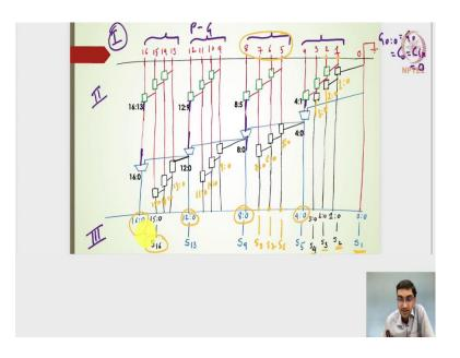
Using this can we now design the PG architecture. The propagate and generate architecture and the first level is nothing but the bitwise, the second one is the group wise where it will generate the group wise generate and group wise propagate bits in this carry skip adder and then the third one is the sum bits generation.
