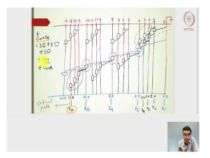
My critical input or rather the critical path which is going to give me the delay expression for this carry skip adder starting from the C input or whenever the inputs are available to see  $S_{16}$  output is nothing but this 3 delay of this 3 boxes plus these 3 multiplexers and then this finally these 3 black boxes and plus of course, the XOR gate and then the PG in the first level in the first stage the bitwise propagate and generate signals delay.
