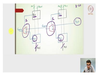
That is why it is called as the carry skip adder. To put this particular multiplexer block into the reality, we have 2 blocks now. One is generating  $P_{4:1}$  from A<sub>4</sub> is to individual A and B input bits. For an 8-bit addition here we have created 2 such blocks one is generating  $P_{4:1}$
