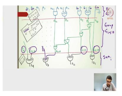
This is what it represents, this level we say that this is the bit level Pi and Gi signals design. This one is the group level  $G_{i-1:0}$  extracting  $G_{i-1:0}$  that is the design for that and last one is our sum bits.
