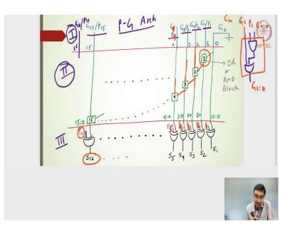
In this particular this is basically the P-G architecture in a very very simple form. Drawing the XOR gates, drawing the OR gates, drawing the AND gates and then drawing the XOR
