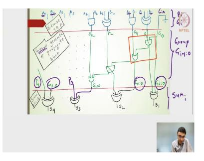
What this diagram the P-G architecture is nothing but it is a very simpler form of representation of the previous AND – OR block space. Here we have the bit wise, group wise and then the sum block. The three stages are now represented by either a straight line or this particular the AND and the AND and OR blocks are represented by a square block in the 2nd stage.
