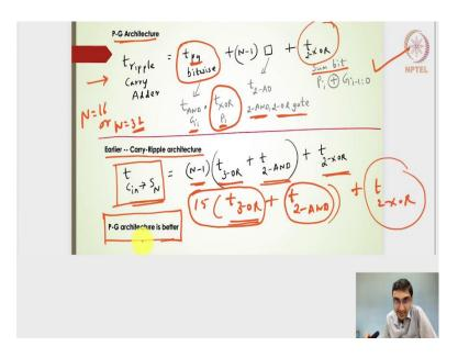
For the P-G architecture the delay for this carry ripple adder is nothing but the P-G bit wise whatever is the delay,
