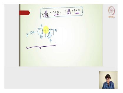
Let us have a look into this particular  $t_{pdq} = 92ps$  and then the  $t_{pcq} = 82ps$ . This is kind of characterized from the latch design and it is nothing to do with the pulse clock or generating signals, because once the pulse signal is given to the latch design, the latch output is my Q signal.
