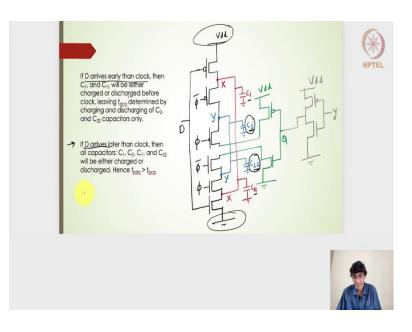
Now, let us say that if the D arrives earlier then the clock, the D signal is given here. The D arrives earlier than the clock, the clock arrives later. This 4 transistors we have the clock signals and let us say that the clock arrives later, but the D arrives earlier.
