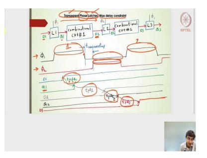
Let us proceed further to the next kind of the sequential elements, which is called as the latches. Generally, latches are not utilized in terms of how we have utilized the flops, the flops are generally utilized for the clock edges with respect to the clock edges. We have the combinatorial circuit design element, within the 2 subsequent flop elements.
