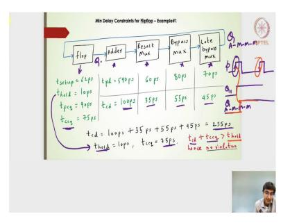
In the last part of the last lecture we had seen this particular design of the flops which is kind of parameterized or characterized with this particular parameters, like the t setup time, the  $t_{hold}$  time, the  $t_{pcq}$  and  $t_{ccq}$ . This is something the sequential circuit or the element characterized elements design is given to us, with all these set of parameters.
