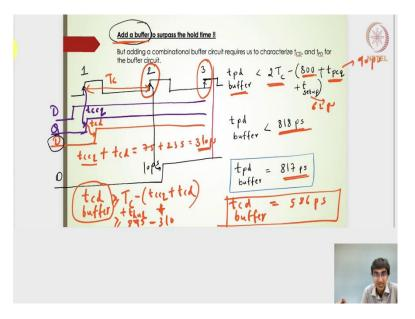
There is another condition here, if I consider the only the contamination delay. If I consider the only the contamination delay. Let me draw the clock here first. I am drawing a very smaller clock this time. This is the 1st edge this is the 2nd edge. I am going to write it as 1 and then this is the  $2^{nd}$  and I want  $t_{ccq}$ .
