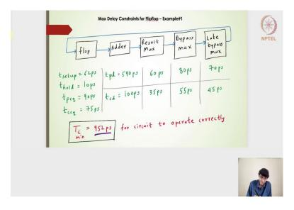
This is what we will get 952ps should be the minimum clock time period, that we do not get into the set of time violation. For the circuit to operate correctly, it should be greater than that. If I choose 100ps that is very well good, that will be better, but it should not go below 952ps.
