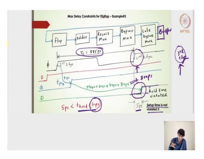
If I do that, this is my clock of 885ps of the duration. The 2nd clock edge is going to arrive after 885ps of the 1st clock edge and if I consider this 90ps of  $t_{pcq}$  and then the remaining this will be our 800ps.
