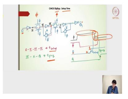
Let us try to understand what is the setup time for the flip flop designs. For the flip flop designs again if I am considering the negative edge flip flop, remember that for the latch design we had considered the positive level of the latch.
