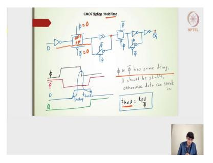
The flip flops again what is the hold time? Again, what we had seen in the latch design is that the D input should stay even after the clock edge going low for the hold time. It should stay at least for a hold time. Even in this case because the  $\phi$  and  $\overline{\phi}$  has some delay, D should be stable otherwise the data can sneak in. The D should be stable or till the hold time has reached and then we will get the expected output.
