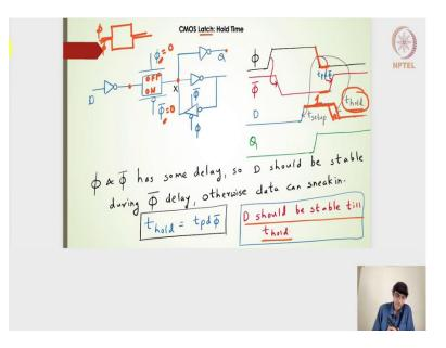
Now, the other significant static timing analysis parameter is the hold time. What is this really the hold time? this is again the latch design which we have been seeing, the most recommended latch design.
