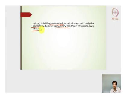
The switching probability assumes the zero  $t_{pd}$  because it always has been defined by the logical functionalities of the gates and it does not accommodate the delays at all. But in circuits when the inputs do not arrive simultaneously. The output transitions will be many times, we will see more frequency of the output transitions and thereby increasing the power dissipation or the energy delivered by the V<sub>dd</sub>.
