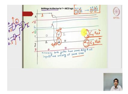
There is one more aspect which we tend to ignore while calculating the switching energy term or the switching power term and let us try to see that in this particular timing analysis. Let us go back to that multi-stage architecture. Again, I am going to draw that multistage architecture. I have two input NAND gate followed by the NOR gate. I will have A B C and D and then here is my x, here is my y, and then this is z, this is my OR gate and then these two are two input NAND gates.
