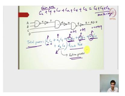
This is what the total power turns out to be. I have an  $f_{clock} V_{dd}^2 \sum \alpha C$  is, which is nothing but alpha for that particular node multiplied by the capacitance at that particular node. If I notice this my  $\alpha_X = 0.1875$ ,  $\alpha_y = 0.1875$ ,  $\alpha_Z = 0.05859$ .
