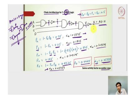
Hello students. Welcome to this lecture where we will continue on the activity factor and using that particular activity factors we will try to evaluate the overall or the average power or the dynamic power, the switching power as well as the switching energy and then the dynamic energy. The last time what we had seen is an output ABCD as a logical expression.
