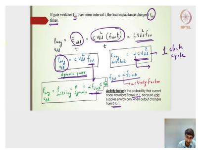
That is what I have rewritten here if the gate switches  $f_{sw}$  times over the time interval t the load capacitance charges  $tf_{sw}$  times. The overall energy that has to be delivered by the  $V_{dd}$  will be nothing but this whole component multiplied by  $CV_{dd}^2$ . That is what I have written
