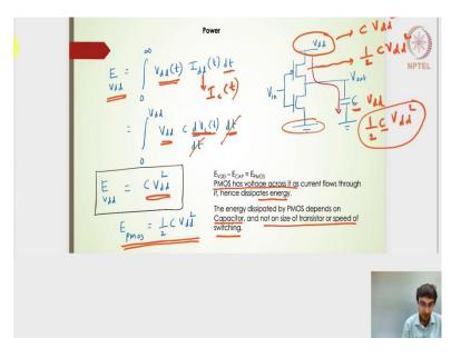
Very interesting to find out that what is actually the energy that will be delivered by the  $V_{dd}$  rail. Now, that is very interesting because the capacitor although it charges to  $V_{dd}$  the energy that it stores or it is consumes will be nothing but  $\frac{1}{2} C V_{dd}^2$  square.
