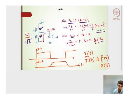
Hope this is clear. Let us take a look at the energy profile and then the power profile with respect to the time domain. What we are really looking into is identifying, what is the power in a transient analysis and what is the energy in a transient analysis.
