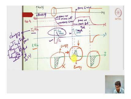
This is what we have, I have an input voltage, it is 0 and then it is the input voltage goes to 1. Whenever it is 0, the output voltage will be 1 steady state voltage and then when it does the transition from 0 to 1, I will get the output voltage doing the transition from 1 to 0. Then while it is doing the transition from 1 to 0 back the output voltage will do the transition from 0 to 1 and then so on.
