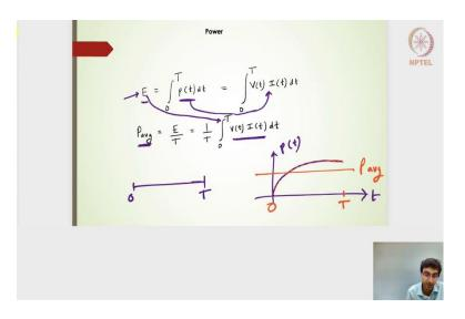
Let us begin further let us move further. Let me take my pointer as well. For the definition for the energy consumed by a particular component or by a particular circuit it is defined as nothing but the instantaneous power that has been consumed by the component or it is been dissipated by the component over a period of time or over a duration of time
