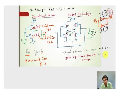
Now let us have a look at the normalized parasitic factor, the normalized parasitic delay in our linear delay model. I am taking an example here of  $24\lambda$  and  $12\lambda$ , let us say that it is nothing but the 6:3 inverter. The 6 inverter represents 6x100nm = 600nm and 3 represents 3x100nm.
