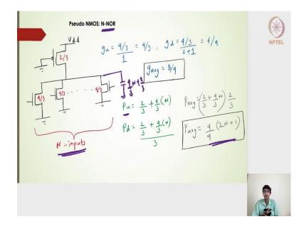
Going ahead, what should be the logical effort for an N input NOR gate, it will be the same  $\frac{2}{3}$  on the PMOS side and then  $\frac{4}{3}$  on all the parallel transistors which are on located on the pull down side.
