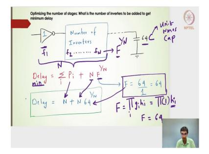
Let us take an example here, we need to optimize the number of stages and what should be the number of inverters to be added to get the minimum delay, the 1st stage is anyways 1. The same example what we had seen in the earlier slide and then we have the 64, what it means is it is actually 64C, where 1C represents the unit NMOS transistors capacitance.
