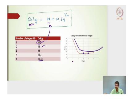
Now, I have the minimum delay expression with the number of stages and if I put a table here, if N = 1, what is the delay if N = 2? What is the delay if N = 3? What is the delay? and so on.
