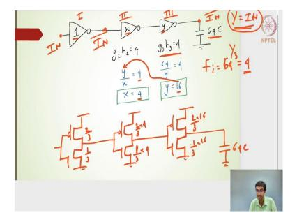
Finally, this is what the circuit will look like. I have the 1st stage, I have the 2nd stage, I have the 3rd stage, 3 stage circuit is going to give me a minimum delay of 15 and minimum normalized delay of 15 for a load capacitance of 64C and then the input gate size of 1. If I want to find out what is the gate size of x and y here, I know the fi value here is nothing but  $64^{\frac{1}{3}}$  turns out which is nothing but 4 here.
