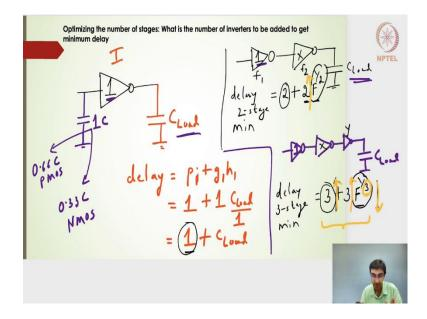
Hello students, welcome to this lecture on trying to learn how to optimize the number of stages for a given circuit, so that we get the minimum delay. Let us begin with one inverter here, the inverter has an input size, let me take input size of 1. What it means is at the input of this particular inverter it sees a capacitance of 1C including both the PMOS and then the NMOS transistors.
