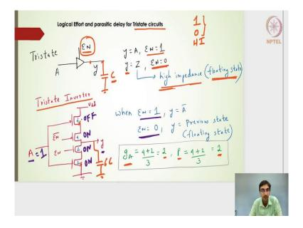
Moving forward, what we will see is a slightly different circuits, although developed from the CMOS families, but it is called as a tristate circuit. What we will do is we will establish the logical effort and then the parasitic delay for a very primitive tristate circuits and then we will go on to the little bit more accomplished circuits.
