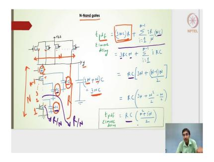
Just to complete the overall the logical efforts and then the parasitic delay. Now basically the linear delay model what I have done here in the next 2 slides including this one will be trying to showcase the Elmore delay model based delay estimation and compare with that of the linear delay model with respect to the number of inputs.
