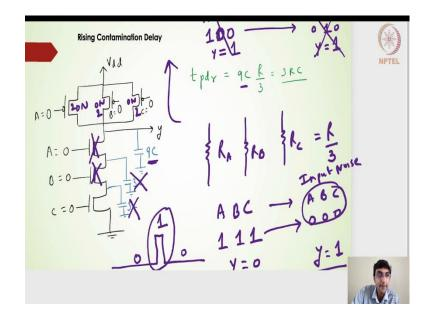
Moving forward, what should be the rising contamination delay. The rising contamination delay is a very straightforward, if all of them I want a rising output here. For always for the propagation delay rising, we are always considered the worst-case where one of the transistor is on, the other two will be off.
