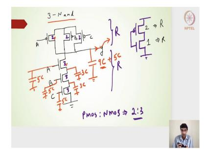
The 3 input NAND gate, I am going to summarize this again. The pull up circuit for the 3 input NAND gate to be in parallel, all the PMOS transistors will be in parallel. This is my PMOS transistors shown with a bubble sign, bubbled input that represents our PMOS transistors.
