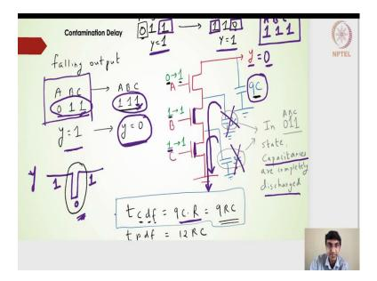
In this particular slide we are going to look at the contamination delay for the 3 input NAND gate. Again, we will look into the falling output, the contamination delay for the falling and the contamination delay for the rising output. Let us take a look at the falling output. What we really want is the input, let us say that it starts from 0 1 1 and then changes to 1 1 0 for a 3 input NAND gate.
