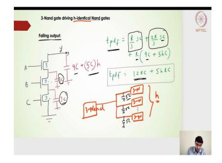
That is what we have in this particular slide, I am talking about a 3 input NAND gate driving h identical NAND gates and what do you mean by the h identical, that means the size of the second stage NAND gates are same. It is basically something like this, the first stage you have a 3 input NAND gate and which is then fed to h such 3 input NAND gate. This the number of the 3 input NAND gate is nothing but h.
