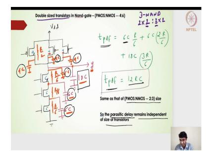
Before getting into p plus dh format I know. Let us see what happens if I change the size of this particular 3 input NAND gate, uniformly scale it. If I double the size of the transistors in the 3 input NAND gate, instead if you remember the PMOS and NMOS in our earlier 3 input NAND gate right. The sizes was 2:3 that means, on the NMOS the size was 3 on the PMOS the size was 2.
