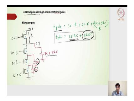
Moving forward what is the propagation delay for the rising output for the same configuration. The 3 input NAND gate driving the h identical NAND gates for the rising output. Again, we will consider the worst case condition is one of the transistor is on and the other two will be off.
