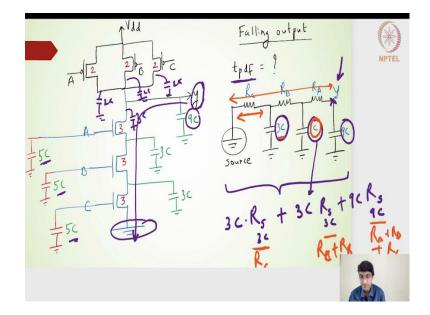
Proceeding further now I have the sizes, now I have the capacitances, now I have the capacitances seen at the output node y which is 9C, I have the gate capacitances which is nothing but overall the pull up and pull down side for the individual inputs turns out to be 5C and then I have the merge capacitance which is nothing but 3C and 3C.
