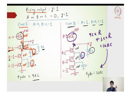
Next, we have to find out the rising output, for the rising outputs because there are three transistors on the PMOS side which are in parallel. What we can have is a three different combinations. Either one of it we can have in fact five different 5, 6, 7 different combinations where the first three combination could be the one of the transistors is on the other two transistors are off.
