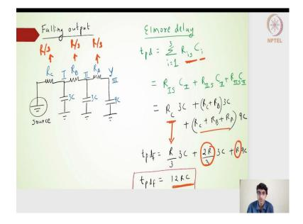
The Elmore delay method for the shared resistance and then the individual capacitance is
