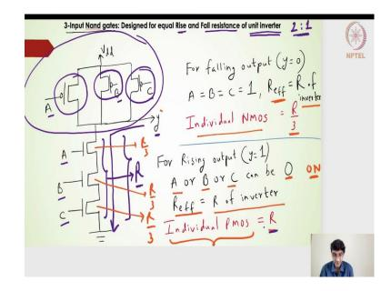
Hello, students. Let us continue with this lecture on the 3-input NAND gates. What we are trying to look into is a 3-input NAND gate schematic and then appropriately find its propagation delay falling as well as the rising delay.
