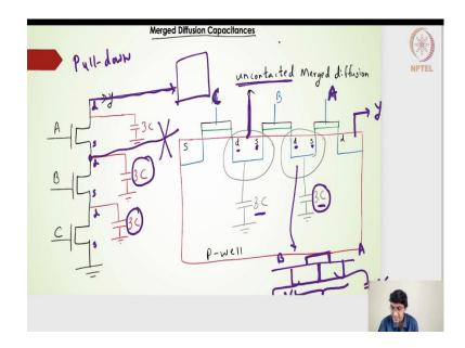
Now, what do we mean by this merged diffusion capacitances, which we had seen earlier, which we had seen in the last slide which is nothing but talking about this 3C and then this 3C. If I draw the cross-sectional diagram of the pull down circuit of the 3-input NAND gate this is what we will get.
