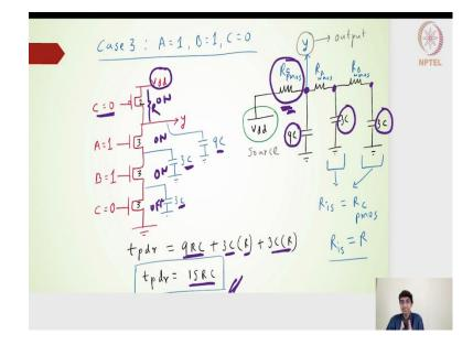
Case 3, when A=B=1, that means C=0, that means this is on in the pull down side and then this is on the pull down side this is off. Now I will have this 3C now, C is a charging path for the  $V_{dd}$  for connecting to the  $V_{dd}$  source. The overall Elmore delay I have written for the charging.
