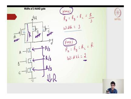
What should be the width of the 3-input NAND gate in that sense, on the NMOS side, on the pull down side we know that all the three transistors which are in series has to be on and then only the y output will get discharged to 0. All the three transistors on the NMOS side has to be on and we had said that each of this transistors should have a individual switching resistance of R/3.
