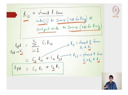
Hope this is clear. Just for a better understanding I have just written it here  $R_{is}$  is nothing but the shared resistance from the node from which the capacitance is connected to all the sources whether it is  $V_{dd}$  or ground, for  $V_{dd}$  for rising ground for falling output and then whatever node is my output node of intersect.
