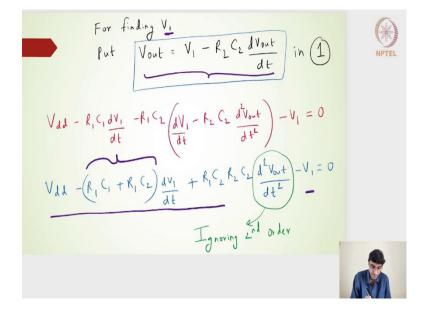
Now, what we are interested is there were two nodes  $V_1$  and  $V_{out}$ . We are also interested in finding out the  $V_1$  and I have two KVL equations written down. What we want is basically from those two KVL equations we want all the terms in  $V_1$ . Whether it would be  $\frac{dV_1}{dt}$ , that is also fine  $V_1$  and then constant that is also fine, but what we do not want is anything  $V_{out}$ . If I go back to this particular starting equations.
