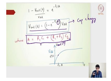
$$1 - \frac{V_{out}(t)}{V_{dd}} = e^{-t/A}$$
