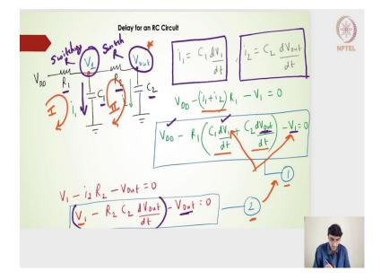
Moving ahead. I have taken a very simple second order RC circuit. I have  $R_1$  and  $C_1$ .  $R_1$  here and then  $C_1$  again cascaded it to  $R_2$  and  $C_2$  and we need to find out the delay of the RC circuit. I have two nodes one is the output node here  $V_{out}$  another one at this point of time I am going to call it as  $V_1$ , there are two nodes  $V_1$  and  $V_{out}$ .
