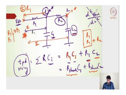
I hope you have understood this or you have analyzed that. Coming back to our original circuit of  $V_{dd}$  and then  $R_1$  and  $C_1$  and then I have this  $C_1$  here and then I have this  $R_2$  and then I have this  $C_2$ . What it says is, the propagation delay rising is nothing but the summation of R into all the node capacitances also called as the leaf capacitances.
