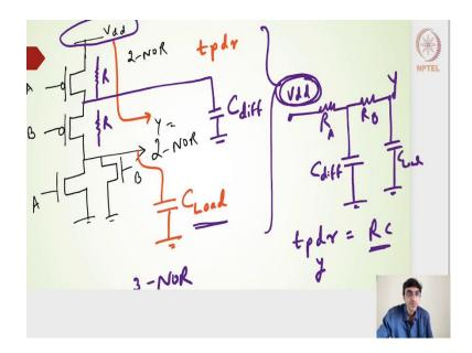
Let me draw a very simple one a 2 input NOR gate. I am going to draw on the PMOS side. This is a 2 input NOR gate connected to the  $V_{dd}$  source and this is a PMOS transistor and then this is my NMOS transistor.
