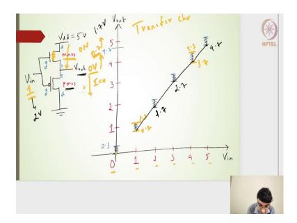
Let us see what it means. If I actually draw a transfer characteristic output voltages with respect to the input voltages. For a specific input voltage in the sense 0 volts or 1 volts or 2 volts 3 volts 4 volts and 5 volts what are those intersection points or what is that output voltage.
