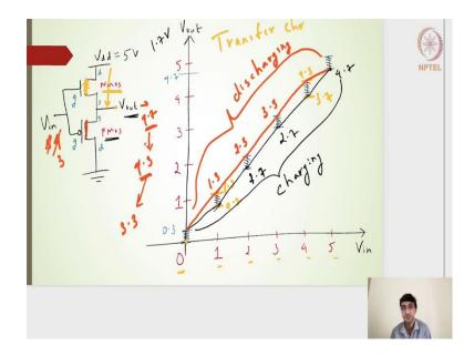
Let us say that the output voltage is 4.7 volts and let us say that the input voltage is 5 volts. In that case my  $V_{gs}$  value is 0.3, whether it is possible for the output voltage to decrease, that cannot, it will have a channel and it starts. The  $V_{gs}$  value is there and it becomes positive, the PMOS will always be off.
