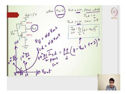
Proceeding further, when  $V_{\rm in}=0$ V, I am taking the extreme case for the PMOS transistor. We started with the PMOS transistor, we started with the input voltage of 5 volts, then 4 volts, 3, 2 and 1 and 0. I am taking the extreme case of 0 volts, I am not taking 3, 2 and 1 volts, because the expressions will be very very similar. I am taking one last extreme case of the input of 0 volts and if this is 0 volts here at the input side.
