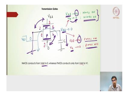
Let us have a look at the transmission gate for the logic 0 passing. On this particular terminal, if I switch off the power supply, I will get again a 0 voltage here. This particular terminal is now connected to the ground and let us say that the capacitor is completely charged to  $V_{dd}$ . For an NMOS whichever potential is higher that will be considered as drain, that is why I have written drain here and then the source here.
