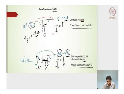
Going forward let us take a look at the PMOS transistor as a pass transistor again. If I look into this, the PMOS transistor again the same thing the gate is connected to the 0 volts because I want the gate to be at a negative potential than that of the source.  $V_{gs}$  value turns out to be negative for the PMOS. I am putting it 0 on both the cases, 0 volts of the gate represents why here it is a gate. 0 volts of the gate represents that the PMOS transistor has a gate potential of 0.
