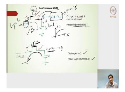
In this particular lecture, what we will talk about is more on the pass transistors and then the transmission gates. I have drawn a pass transistor here. In this particular case, it is a pass transistor means a single transistor, and I have considered the NMOS as the pass transistor here and then we need to understand the working of this particular NMOS transistors. The pass transistors can also be designed using the PMOS transistors and that is something we will see in the future slides.
