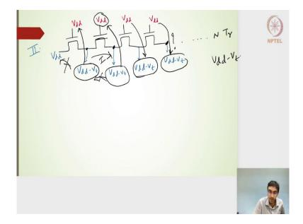
Second configuration where we have again a cascaded one, I call it as a stacked 1 and then this one is called as a cascaded 1. The reason is nothing but the output is connected to the input of the pass transistor and again the output of the second transistor is connected as an input to the third transistor and so on. Finally after four transistors cascaded four transistors configuration what should be the output here?
