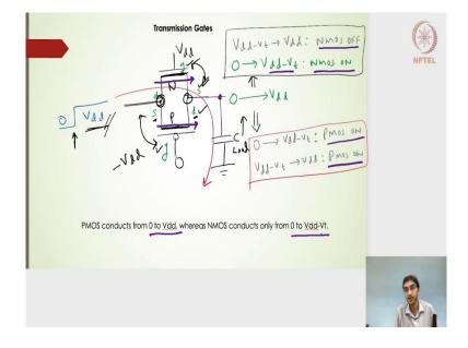
Moving ahead now let us take a look at the transmission gates. Alright, earlier we had seen the series the inverter which is nothing but a series of the PMOS and NMOS transistors. Here instead of having a series of PMOS and NMOS transistors, what we have is a parallel combination of PMOS and NMOS transistors. I have a PMOS transistor this one the bubbled gate shows that is a PMOS transistor and the unbubbled gate is an NMOS transistor.
