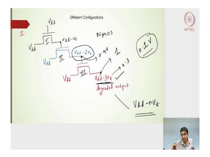
I have drawn two different configurations here. One where we have a stacked transistors and the output of this particular first transistor is connected as a gate to the next transistor. The next transistor output is connected to the third transistor. In this particular configurations I have three transistors and then we have the supply of  $V_{dd}$ .
