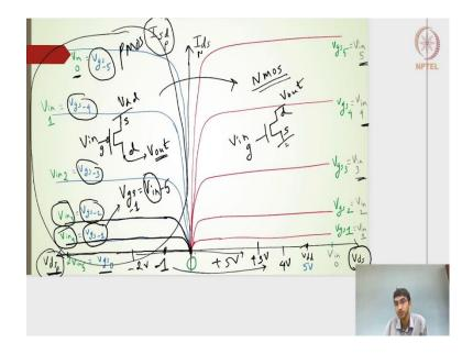
In the last lecture we had seen the NMOS. As an inverter, the NMOS and the PMOS transistors in series and if you want to find out the solutions graphically, you know the way we wanted to do graphically is to avoid understanding of whether it is in saturation region or linear region.
