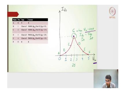
So, that is something we will see it now and then this is again another profile of  $I_{ds}$  with respect to input voltage. So, the earlier one was  $I_{ds}$  with respect to output voltage. So, I have drawn with respect to the input voltages those series of points A, B, C and then D, E, F and then this is one point G point, where the input is 2.5 volts and where I will have the NMOS and PMOS saturation current to be equated.
