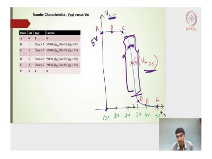
And then, this is the last one is the transfer characteristics, where we have the output voltage drawn with respect to the input voltage. So, I now have the points A, B, C, D, E,
