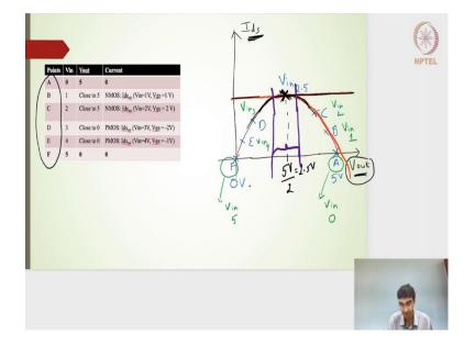
Moving ahead if I want to draw now, that we have this particular intersection points A B C, D, E, F and then it is the current value, it is input to voltage, is output voltage. Although we do not know the real output voltage graphically, we can only say, that it is close to 5 volts or close to 0 volts.
