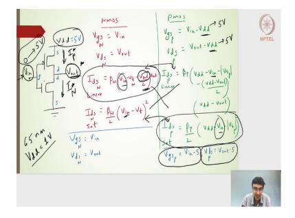
Coming back to this particular slide of the inverter, where we had the PMOS and NMOS in series. This particular  $V_{dd}$  let us for time being let us say that we will fix it to 5 volts. Generally for a 65 nanometer technology node which we will generally use, the  $V_{dd}$  values are generally 1 volts not more than that. Maximum of it will go to 1.2. The minimum it might go is 0.8 volts.
