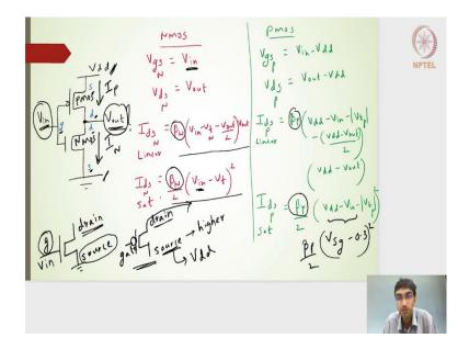
The inverter is, as you may be knowing it is formed of the NMOS transistor and then the PMOS transistor. This is one such circuit where the PMOS is there, PMOS is in series with of the NMOS and where the PMOS is connected to the  $V_{dd}$  rail.  $V_{dd}$  represents a higher
