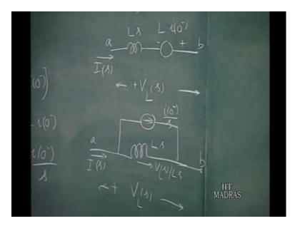
We can think of that having a generalization impedance Ls and we have a current passing through it not the raw current, but the transformed current Laplace transform variable and across the terminals of inductor we must away among voltage of VL of s. So, this is the voltage of the terminals of that we know, that VL of s is the Ls times i of s minus L i 0 minus.
