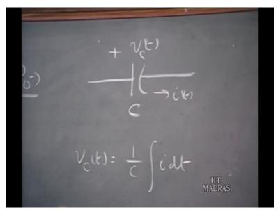
And we can make use of this, when suppose have a capacitor value c and this is the voltage across the capacitor vct and the current the capacitor is it then we can write vct is 1 over c the integral of the current which is the charge or the capacitor.
