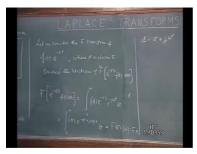
To do that let us consider the Fourier Transform of not f of t but, f of t multiplied by e to the power of minus sigma t. So given a f of t we do not find the Laplace Transform, we will not find the Fourier Transform of that as such. Let us consider f of t e to the power of minus sigma t where, sigma is chosen to ensure the existence of the Fourier Transform of e to the power of minus sigma t f of t.
