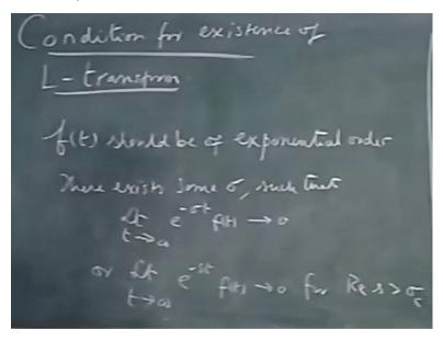
This condition is usually stated as: f of t should be of exponential order. In other words, f of t cannot grow with positive t more than, an exponent of some value or in other words, there exist some sigma real value such that, limit as t goes to infinity of e to the power of minus sigma t f of t goes to 0. So, there must be some real value sigma such that, as t
