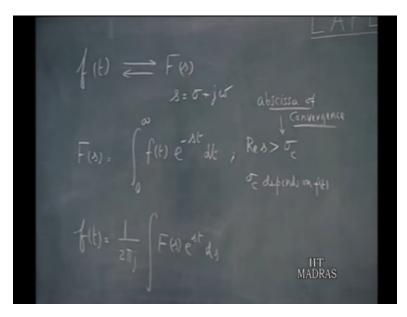
So, given any function f of t, we will indicate its Laplace Transformation as F of s where, s is the complex frequency variable which is real part sigma and imaginary part omega. And so we indicate the a function of time and Laplace Transform pair in this manner. F of s is obtained from a given f of t by this defining integral 0 to infinity of f of t e to the power of minus st dt and this is called the Laplace Transform integral.
