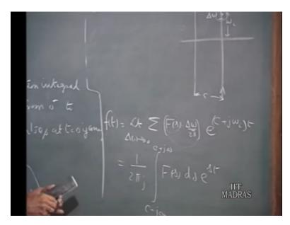
A third point which we like to notice: that in the complex frequency plane this is the Bromwich contour and we are taking the integration along this and so as you move along this line, you are incrementing omega. So you can say, you can divide this entire contour into small intervals of width delta omega and suppose, you have the centre point is omega i then, we can think of f of t as composed of elementary exponential signals of the form; e to the power of sigma.
