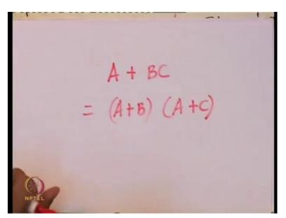
So, what the thing that I am using is, I am using this theorem which is essentially a plus b c is the same as a plus b into a plus c. So, this is the theorem that I have used to expand to the first line.
