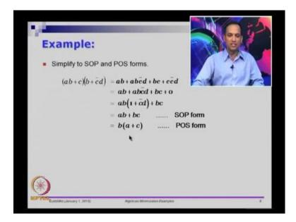
So, let us look at this example, simplify to SOP and POS forms. So, let us say, I have a b plus c into b plus c bar d. So, this is clearly not in the SOP form, nor in the POS form. So, it is neither of those, we want to convert that both SOP and POS form. So, if you are asked a question like this convert to both SOP and POS form. So, first thing you have to do is, get it in one form, so let us try and get it in the SOP form first.
