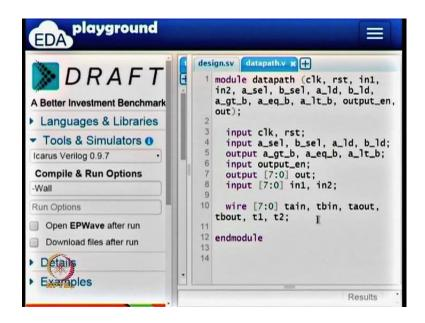
The data path again will have 2 inputs. So, there are 2 inputs, input 7 colon 0, input 1 and input 2. So, here this is the data and I miss that. So, again now let us go and look at the picture for the data path itself. ((Refer time: 16:09)) So, we have several things here. So, we have two subtractors, three registers, one comparator and two multiplexers, but before we get it to what these are, we need a few more things.
