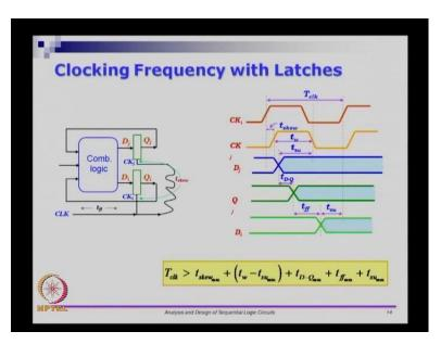
What I want to show is the clocking frequency with latches, so let us look at the circuit here, here these are not flip flops these are latches and we have a circuit like before except that these two are latches. So, I want to know drive the relationship for clock frequency of latches. So, we have various signals here, we are CK i, CK j, D j to Q j, so and D i. So, we have several data inputs, so D j, Q j, D i and so on I want to look at the relationship between various parameters.
