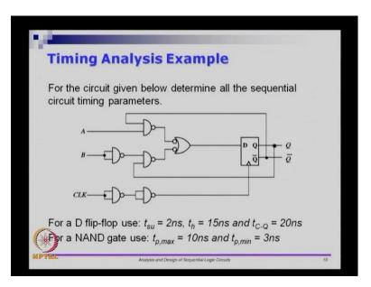
Let us do a small example, so we have a circuit it is not worry about what the circuit does there are two external inputs A and B and this an external input called clock and we are looking at what is the time at which the we want to do the timing analysis of this circuit, we want to look at various timing parameters like t s u, t h what is a frequency at which we can run and so on.
